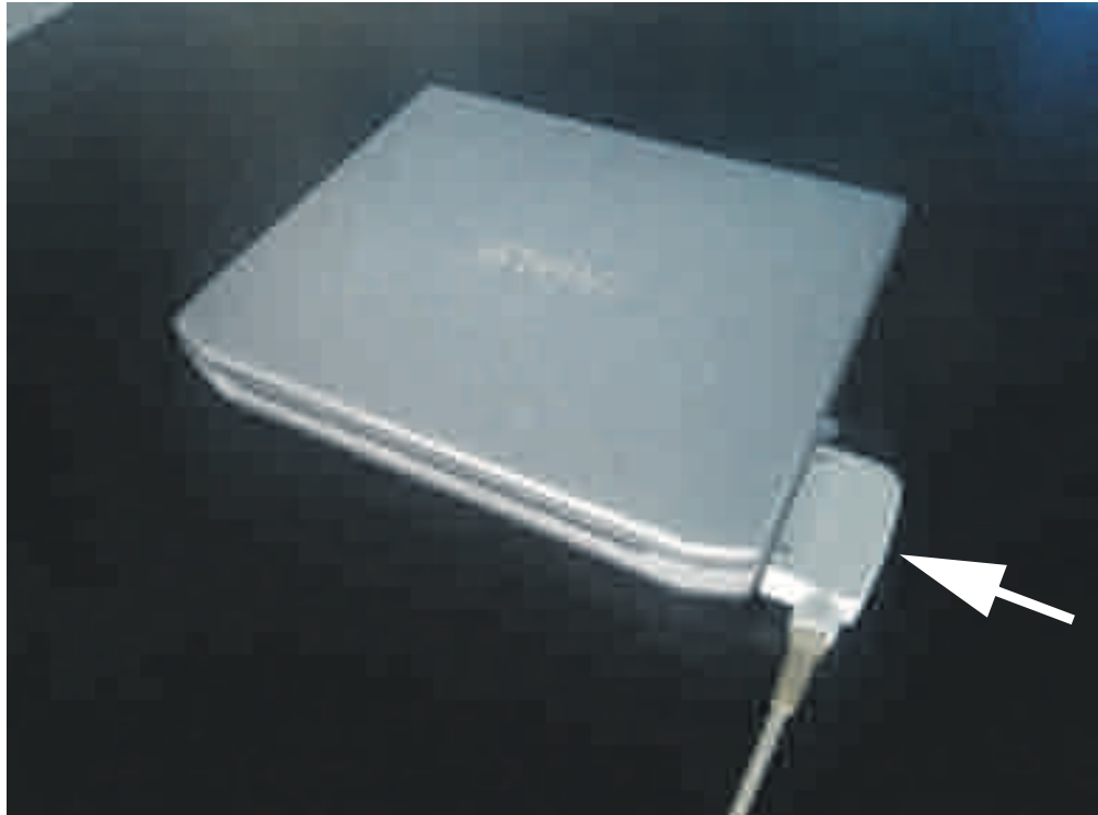
Figure 3-4: Probe Connection to the Unit
