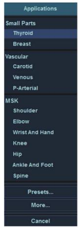
**STEP 4** Move the trackball to the desired application.
