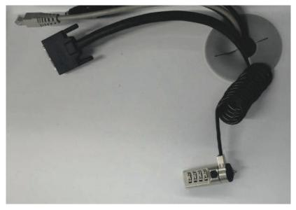
Figure 6-11: The combination cable lock
